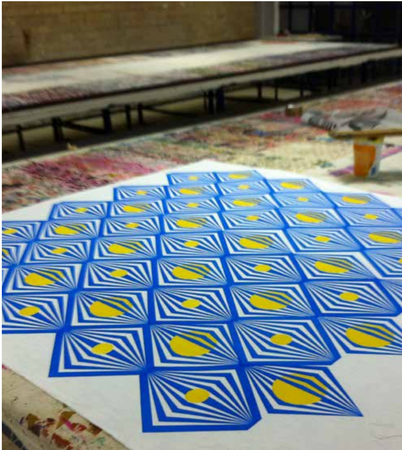
Patterns printed in 100% cotton gabardine with screen printing. Preparation of frames for screen printing and water based inks.
